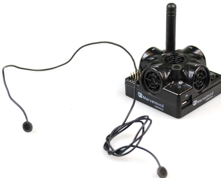
Figure 3 Super-Beacon with two external microphones connected
