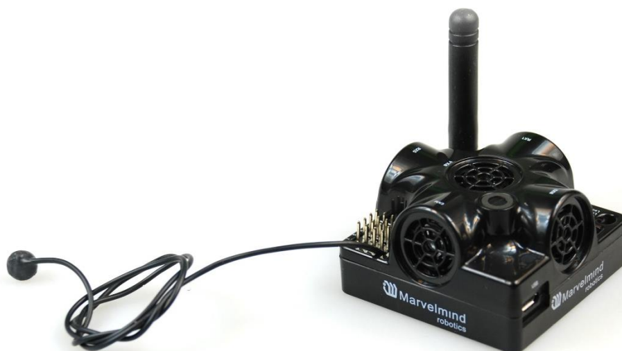
Figure 2 Super-Beacon with one external microphone connected
